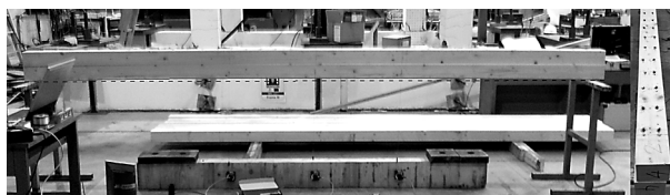
Fig. 3. Composite beam C1 after fastener insertion (starting from the beam centre)
