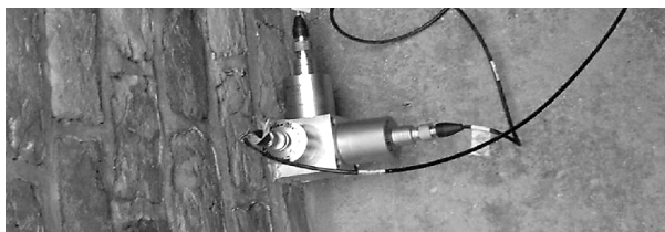
Fig. 10. A triaxial measuring system made up by three DeltaTron 8340 accelerometers
