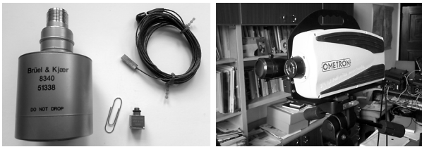
Fig. 2. A seismic accelerometer DeltaTron 8340, mini-accelerometer THETASHEAR 4507, PCB dynamic strain gauge (on the left) and Laser Doppler Vibrometer (on the right)
