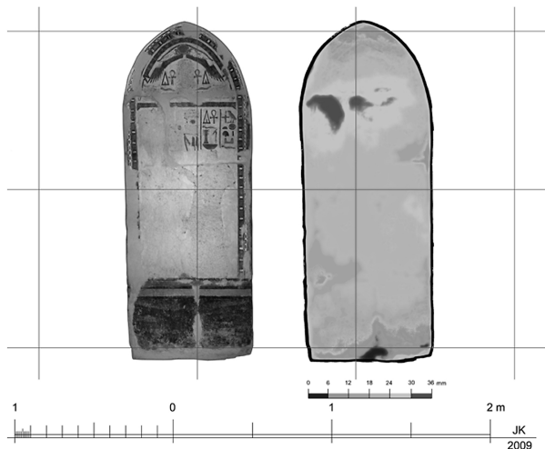
Fig. 7. Example of displacement map delivered directly from 3D point cloud. Southern wall of Upper Anubis Shrine in Hatshepsut Temple in Deir el Bahari (Egypt)
