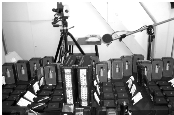
Fig. 1. Brüel & Kjær's PULSE system with 34 measure channels
