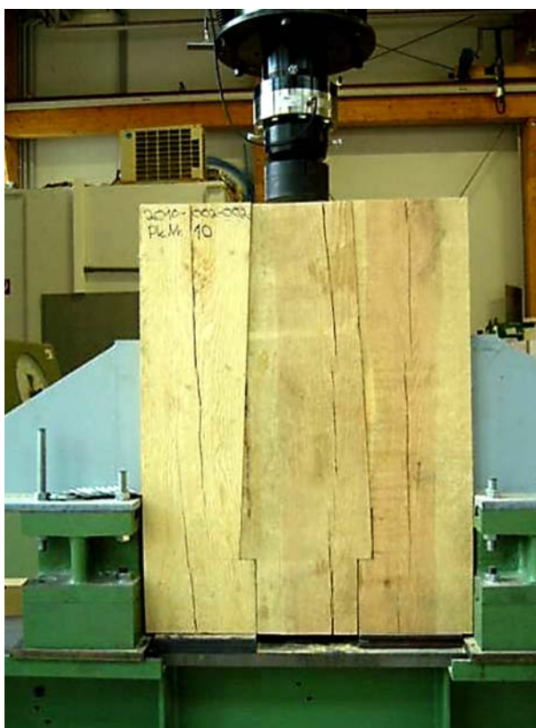
Fig. 5. Specimen (scale 1:1) for the determination of the load bearing capacity and the load-deferral behavior
