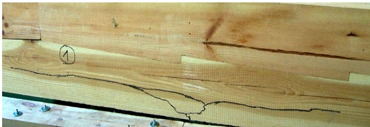
Fig. 12. Specimen 01 – brittle fracture in the sapwood and horizontal cracks in the heartwood
