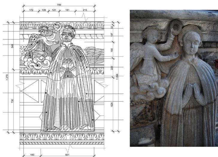
Fig. 7. Black House on Rynok Square in Lviv, sculpture of St. Stanislaus, damage cartogram of losses by O. Rybchynskiy and M. Hohon, 2019; photo by O. Rybchynskiy.
